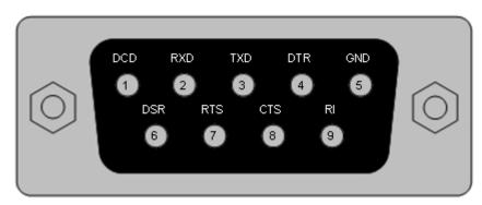
Figure 3-1 RS232 DB9 Pin Out
