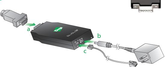
NOTE: Once power is connected, the lights will blink while the system boots up and the red power light will blink until the IP address is assigned.
